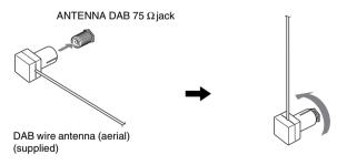
Connect a DAB external antenna (aerial) (not supplied) to the ANTENNA DAB 75  $\Omega$  jack on the rear of the unit.
